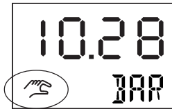
Fig.: Display after switching to the manual mode
